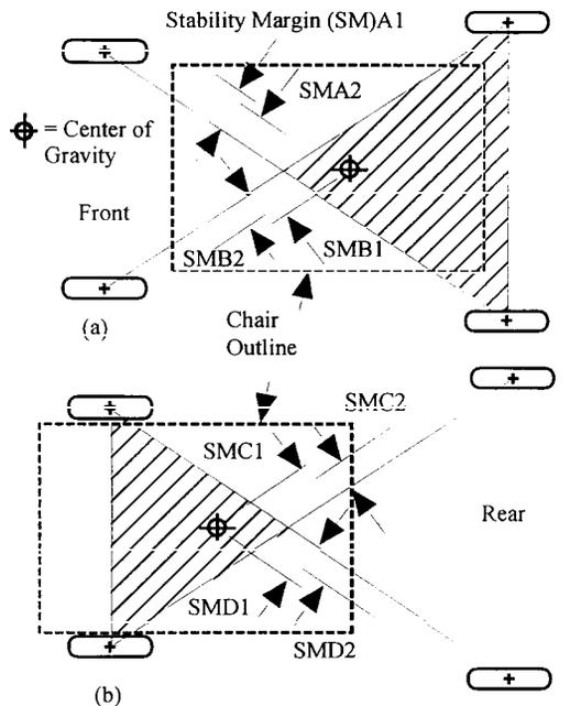
Stability Margins A-D1 = SM with wheel on the ground
