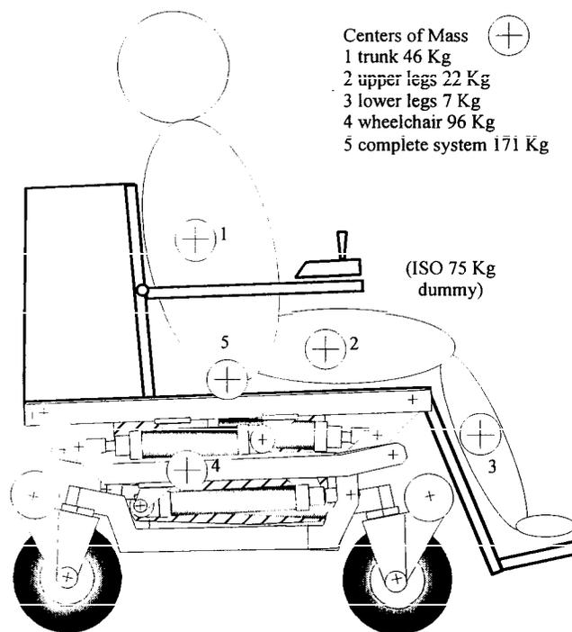
Fig. 1. Proposed wheelchair design side view
