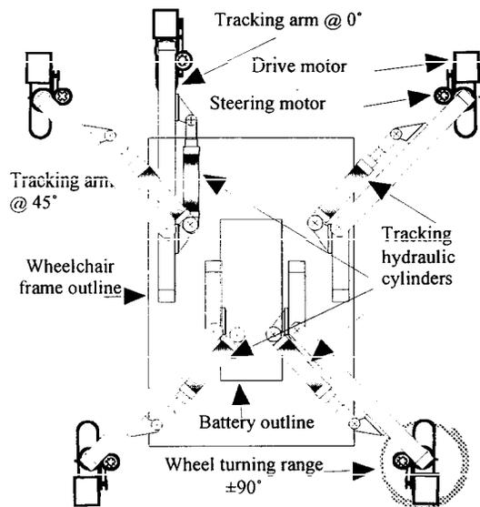
Fig 5. Plan view of wheelchair in maximum tracking mode
