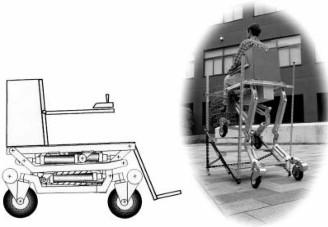
**Figure 3.** Mk2 stairclimbing wheelchair
