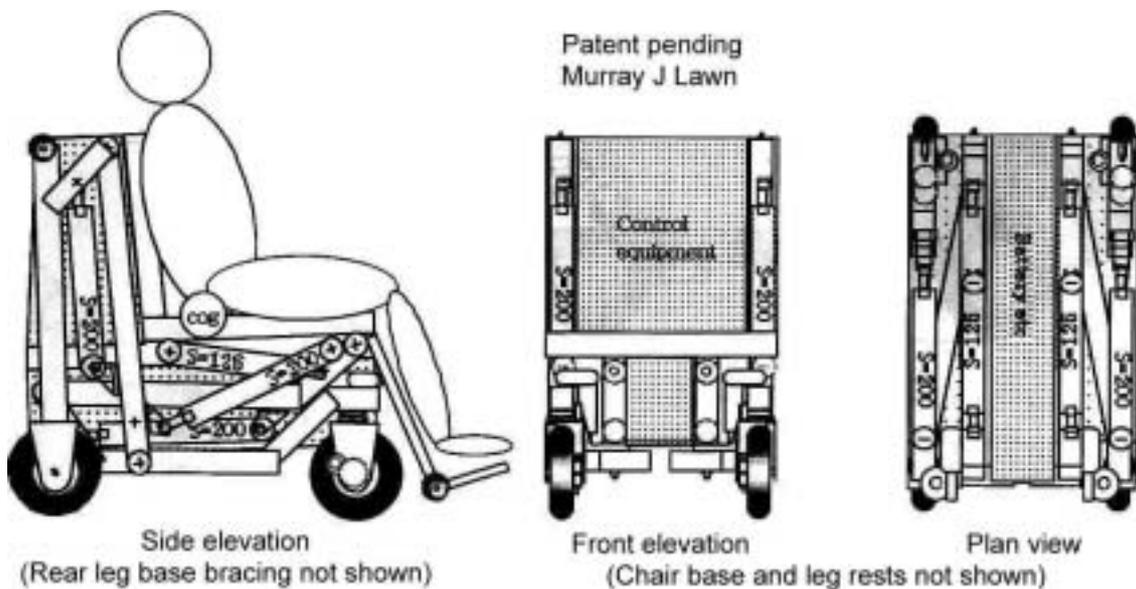
**Figure 2.** The concept barrier free wheelchair
