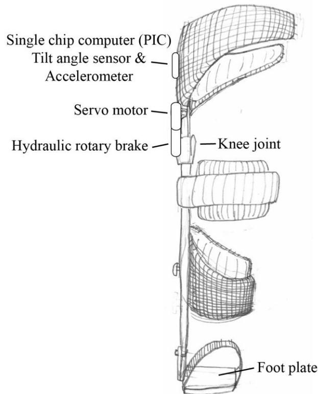
Fig. 2. Orthosis made from carbon material (Tepex®) and control mechanism
