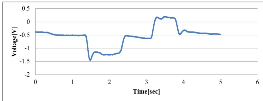
Fig.8 EOG signals obtained through vertical movement of the eye-ball
