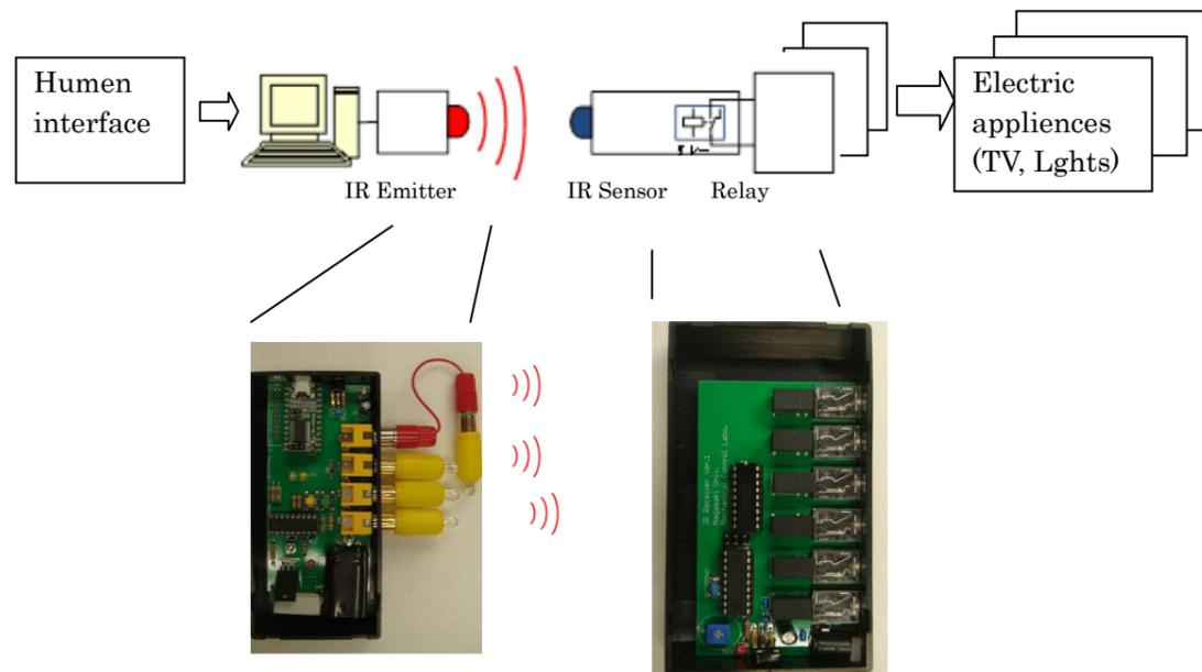
Fig.3 Infrared emitter and receiver
