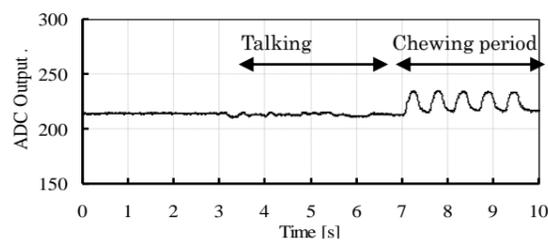
Fig.5 Chewing signal detected by capacitance sensor
