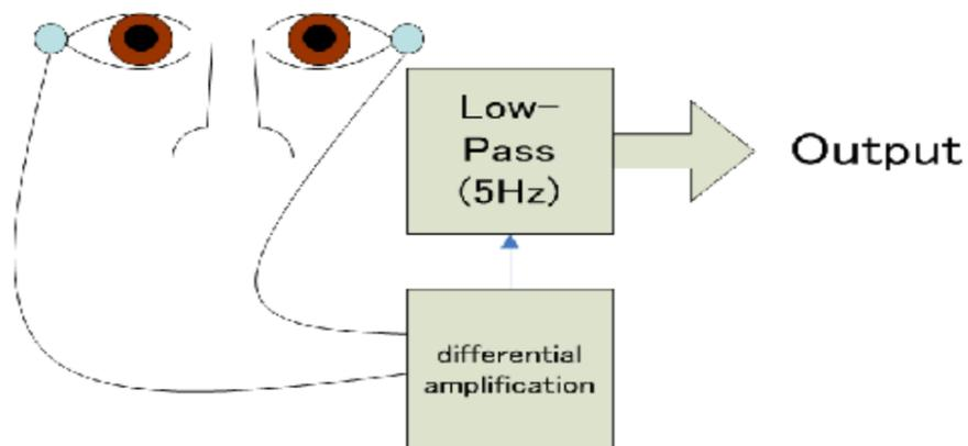
Fig.6 EOG signal obtained by differential aplifier
